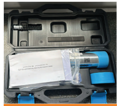
4.) Concrete Test Hammer (Schmidt Hammer) N type
