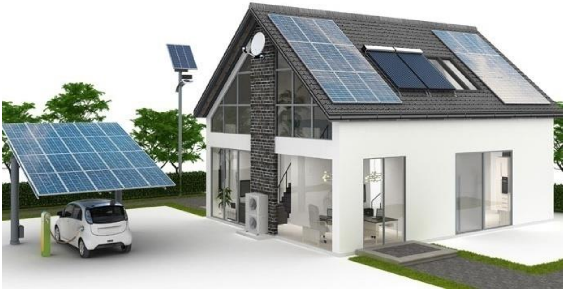
Photovoltaic panels and Hot water solar heating panels
