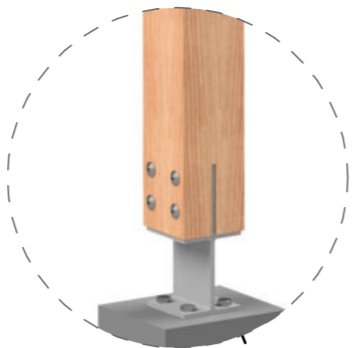
VERTICAL ENGINEERED TIMBER FINIS
